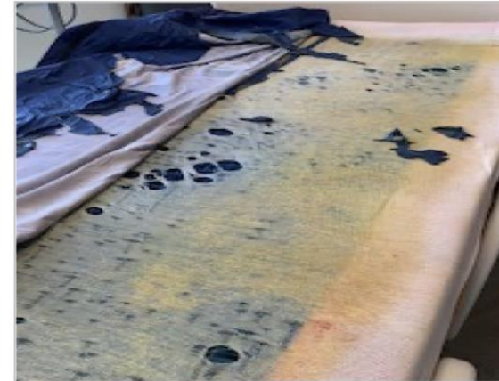
Inside of top mattress cover is DISINTEGRATED BY DISINFECTANT use as well as fire barrier sock protecting the patient.
