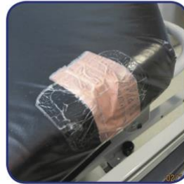
Damage larger than four inches
