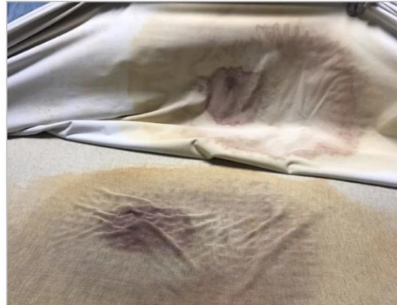
Fluid emersion INSIDE mattress, staining on bottom of top cover, fire barrier, & foam.
